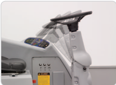
Ergonomic command compartment with tilt steering allows for easy boarding.
