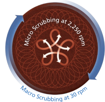
Patent-pending REV random orbital scrubbing technology with high-speed, 1/4-inch micro scrubbing and rotational, low-speed macro scrubbing attacks dirt from multiple directions for superior cleaning effectiveness.
