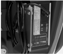
Standard onboard battery charger for wet or gel battery packages.
