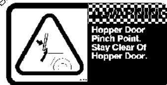
HOPPER DOOR LABEL - Located below the hopper door.
